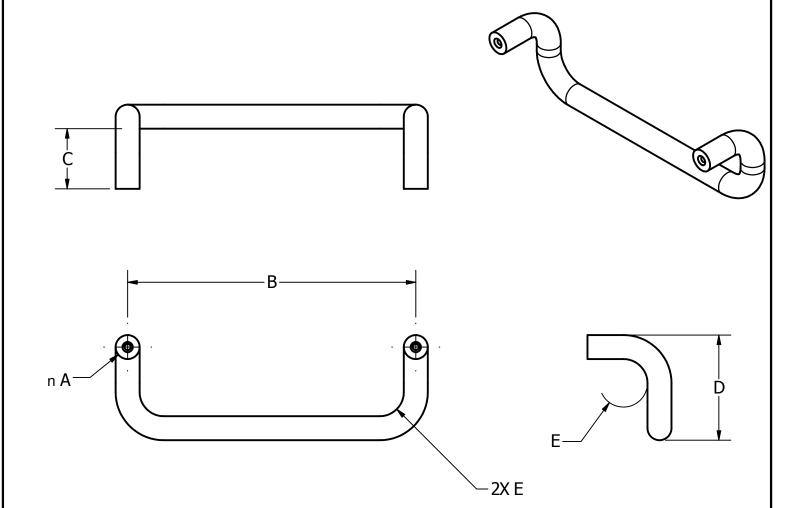
SUPPLIED WITH TWO 5/16-18 SPANNER CAP, FLOW THRU BUTTONS
