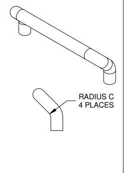
SUPPLIED WITH TWO (2) 5/16-18 X 2.5 FLAT HEAD, PHILIPS DRIVE MACHINE SCREWS AND TWO (2) FINISH WASHERS
