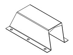
\*\*\*PG8125VV-1 IS AS DRAWN, WITH 6 MOUNITNG HOLES. HOWEVER, PG8125VV-4 ONLY HAS 4 HOLES, THERE ARE NO MIDDLE HOLES ON PG8125VV-4.
