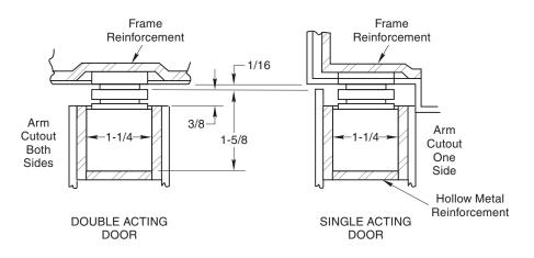
4. Locate "C" and "E" dimensions on top of door and mortise 3/8" deep as shown for arm cutout.
