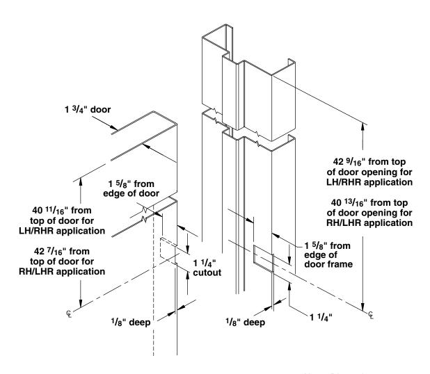
**Note:** Dimensions are true based on industry standard of 1/8" clearance between top of door opening and top of door.
