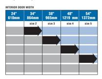
NOTE: Size 1 meets ADA accessibility requirements (5 lbs. maximum opening force for interior doors). Please contact customer service for door weight and size limits.
