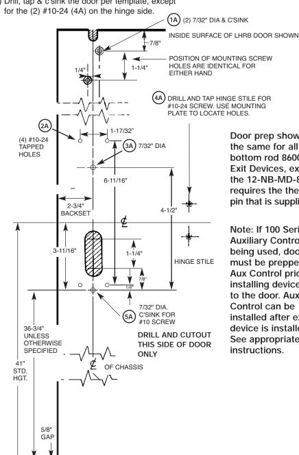
Door prep shown is the same for all less bottom rod 8600 Exit Devices, except the 12-NB-MD-8600 requires the thermal pin that is supplied.
