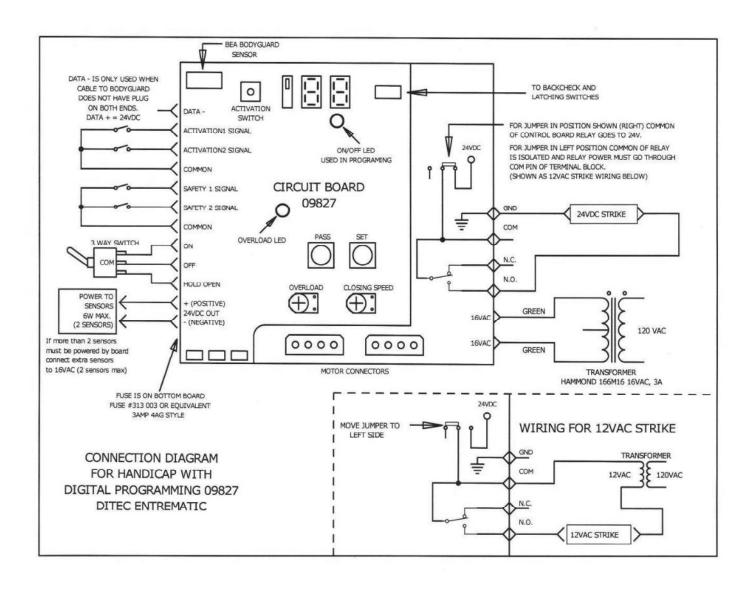
**Note**: A Switch or Jumper must be wired from the ON terminal to the OFF terminal for Programming to work. This is only needed if there is no switch on the board.
