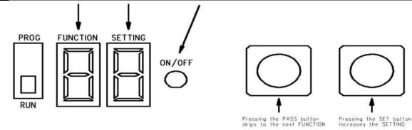
RESET TO DEFAULT - Pressing both the SET and PASS buttons together, for 5 seconds, will reset the product to its original default settings.
