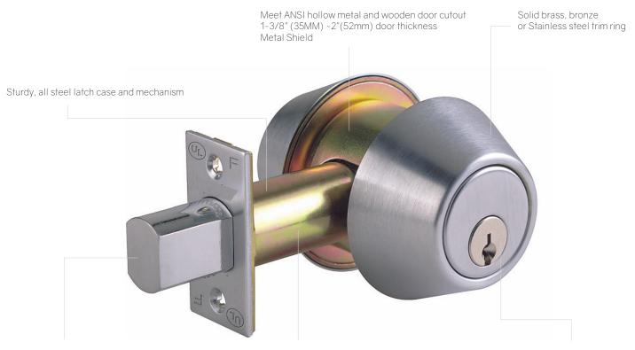
Solid Brass 1" (25.4mm) throw with hardened steel pin inserted Reversible latch for flat & beveled door UL Label UL 3 Hour fire rated Precision solid brass pin tumbler cylinders cap-nut way with brass keys Schlage "C" keyway, Weiser & SFIC available
